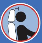
The head restraint is used to prevent whiplash and resulting neck injuries. The driver's head should be no more than 21/2 inches away from the head restraint. The back of the head touching the head restraint is OK.
