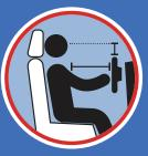
The steering wheel should be adjusted so its center (which contains the airbag) is aimed toward the driver's chest or torso.
